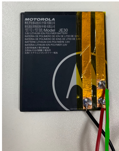
Figure 10: Solder the exposed terminals.
