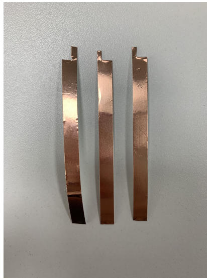
Figure 6: Cut 3 pieces of copper tape.
