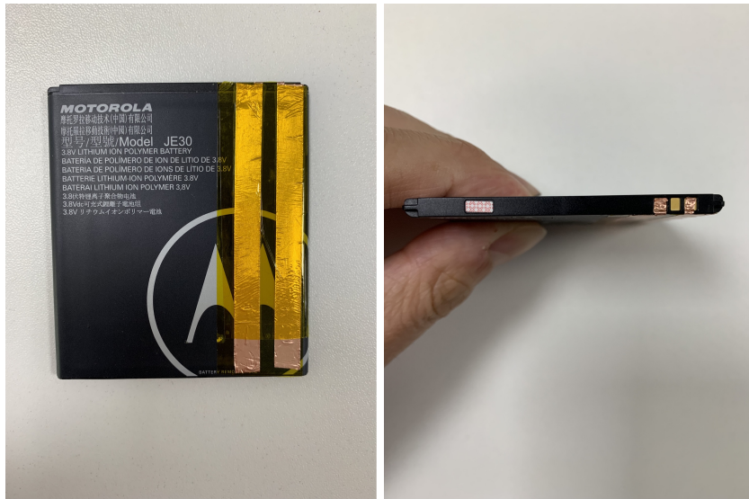
Figure 7: Install the two copper tapes and secure them with Kapton tape.
