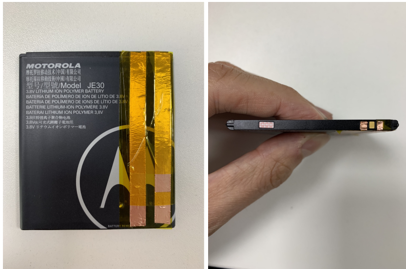
Figure 9: Install the 3rd copper tape and secure it with Kapton tape.
