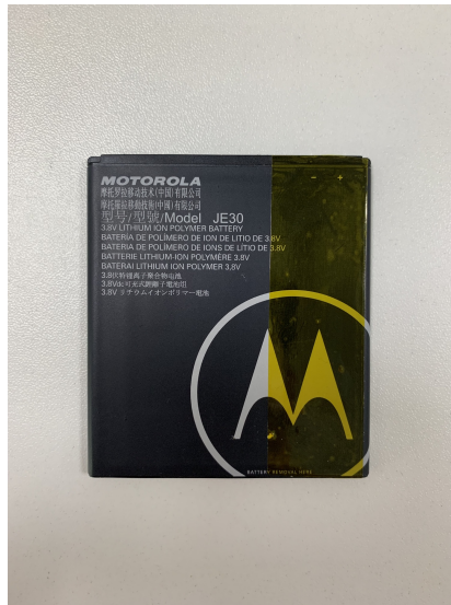
Figure 5: Cover the top side of the battery with some Kapton tape.
