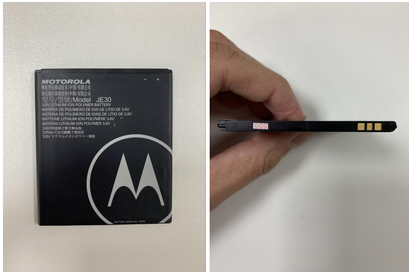
Figure 4: Locate the battery's Voltage (+) and Ground (-) terminals.
